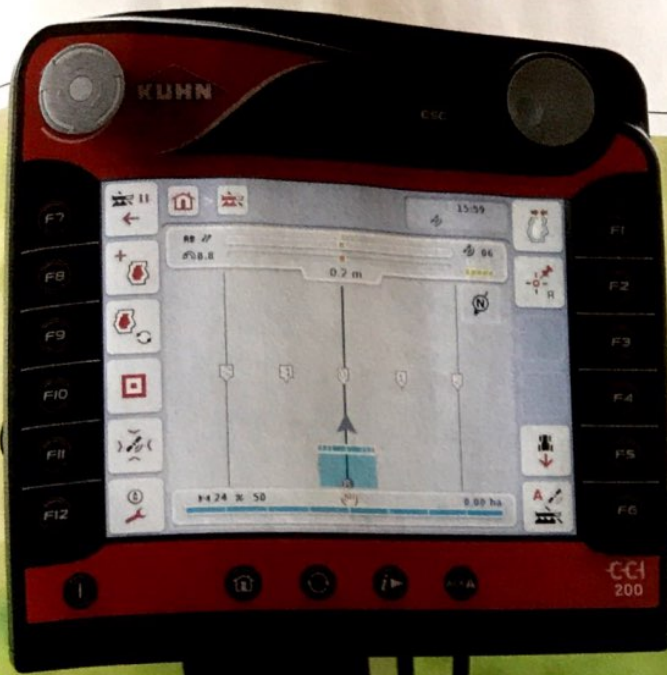
Kuhn's CCI 200 IsoBus terminal uses data from variable rate maps.
